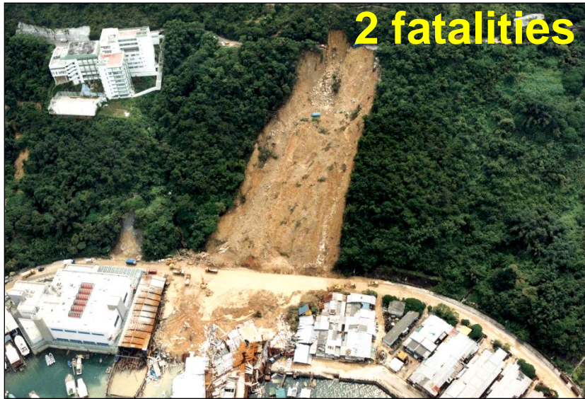
1995 Shum Wan Rd Landslide (26,000 m 3 )
